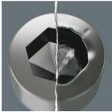
Hexagon screws can endure a problem because the contact surfaces delivering the power from conventional tool, is transferred to the screw via very small surface areas. consequence: the screw can become damaged (rounding out). Hex-Plus tools have a greater contact surface that prevents this from happening! At the same time, as much as 20 % more torque can be applied. Good to know: Hex-Plus tools fit into every standard hexagon socket screw!
